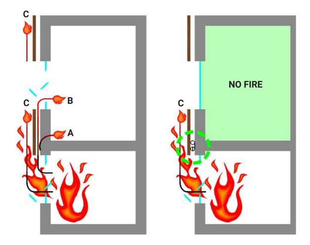
As the FBH prevents any concealed fire in the cavity, the only way for fire to spread is on the panels' outer surfaces (C). Flames (C) are no longer supported by the torch (B) emanating from vent opening at top of air gap so its capability of leap frogging to next panel is significantly reduced.
