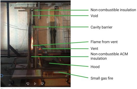
Figure 34 - Cavity barrier test rig
