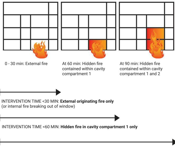
INTERVENTION TIME <90 MIN: Hidden fire in cavity compartment 1 and 2 only
